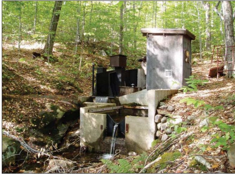
Figure 5. The V-notch weir at Watershed 6 of the Hubbard Brook Experimental Forest, NH. The long-term stream chemistry monitoring data shown in Figure 4 are from this stream.
