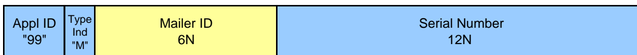
Figure 12. Field Layout of the Intelligent Mail Container Barcode with 6-Digit Mailer ID
