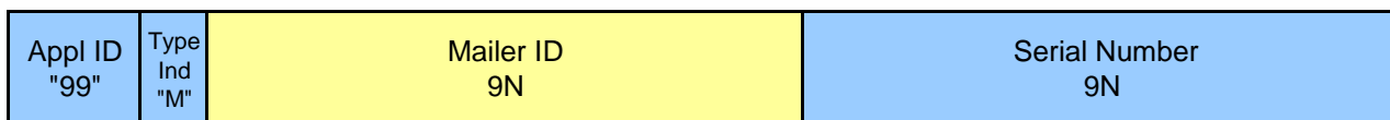
Figure 11. Field Layout of the Intelligent Mail Container Barcode with 9-Digit Mailer ID
