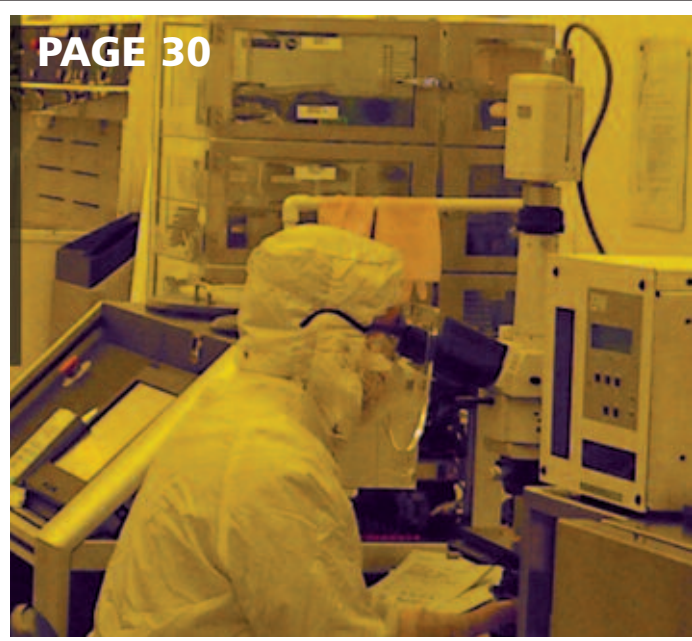
A NASA EMPLOYEE WORKS WITH THE MASK ALIGNERS AND WAFER BONDER AT GODDARD SPACE FLIGHT CENTER'S DETECTOR SYSTEMS FACILITY. THESE LABS AT GSFC ARE AVAILABLE FOR USE BY OTHER GOVERNMENT, ACADEMIC OR COMMERCIAL ENTITIES.
