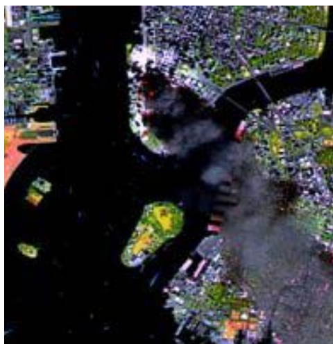
FIGURE 6.9 SPOT multi-spectral image with 20 m resolution taken 87 minutes after the collapse of the North Tower of the World Trade Center (WTC) and 110 minutes after the collapse of the WTC South Tower, clearly showing the particle plume transport to the SE. Approximately 3 km from the source, the visible plume is about 1 km wide. (SPOT image © CNES/SPOT 2001)
