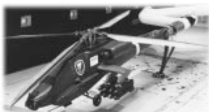
Rotorcraft model with 3-joint rotary sting.
