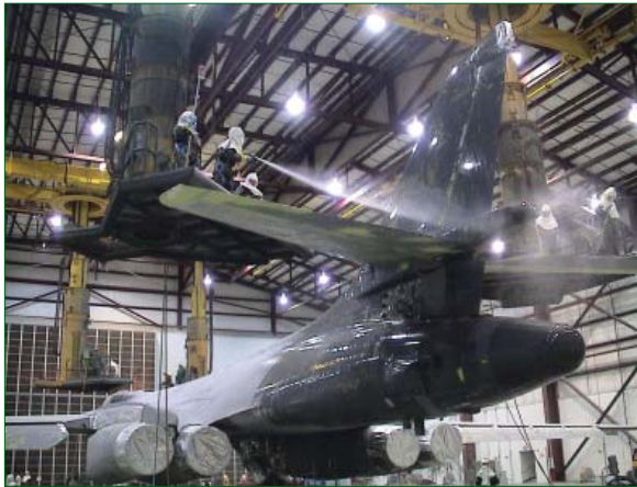
Tinker Air Force Base converted the B-1, B-52, and C-130 aircraft surface treatments to a more environmentally sound process, saving $120,000 annually and resulting in better paint adhesion.
