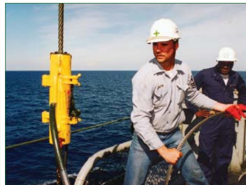
Pollution Prevention Afloat Team developed a cable lubrication technology that reduces pollution and provides greater safety for Sailors and the environment.
