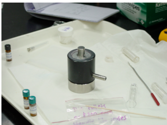
Figure 7: Put the Plunger into the Die Barrel on top of the Bottom Pellet
