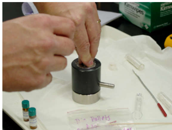
Figure 6: Insert the Top Pellet into the Die Barrel with the shiny side DOWN.
