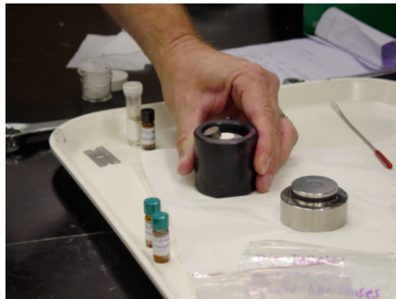
Figure 11: Invert the Pellet Die Assemble and press down gently on the Piston. The Bottom Pellet and the pressed Sample Disk should pop out.
