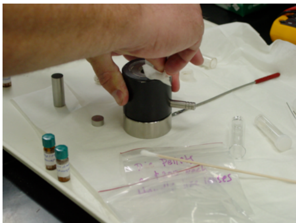
Figure 5: Level the sample in the bore and wipe off any spilled powder.
