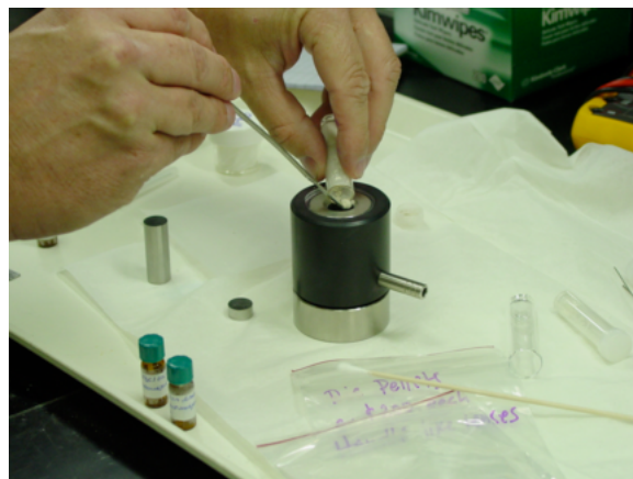
Figure 4: Pour your powder into the bore of the Die Barrel.
