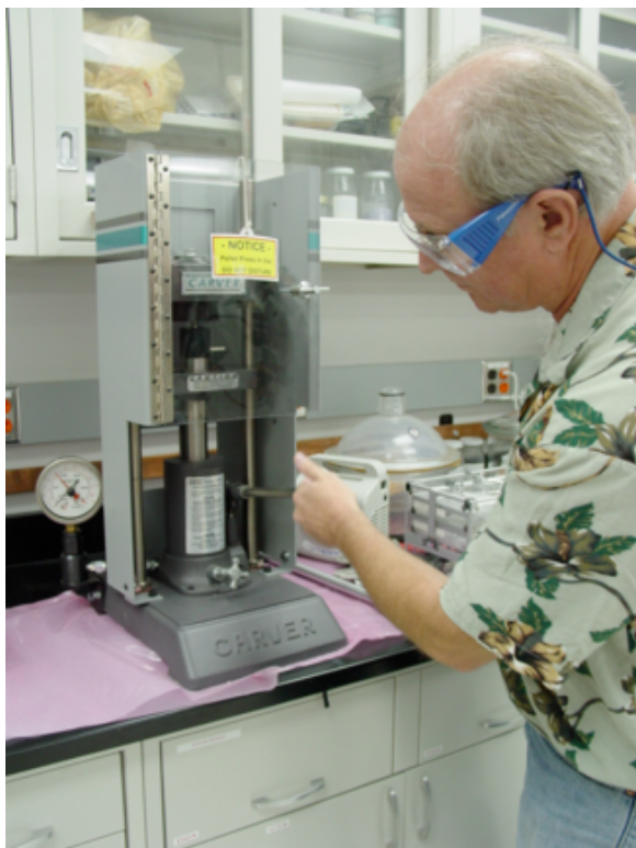
Figure 8: Center the assembled Pellet Die on the platform in the Pneumatic Press.
