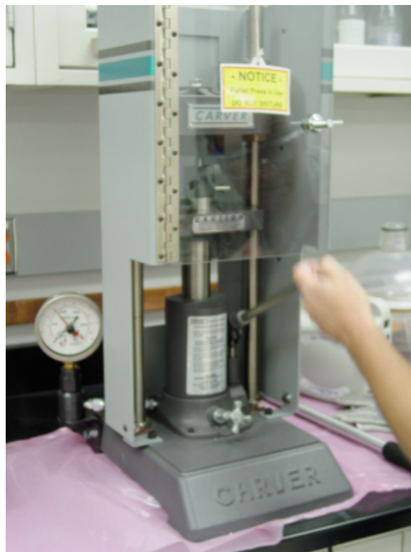
Figure 9: Pump the handle to raise the lower platform.
