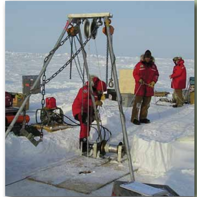
Re-deployment of the North Pole Environmental Observatory (NPEO) mooring in 2004. The hydraulic power pack is seen on the left through the quadrupod legs with hoses connected to the capstan in the lower center. The deployment hole through the ice is covered except when large items are passed through. From Aagaard and Johnson (2011)
