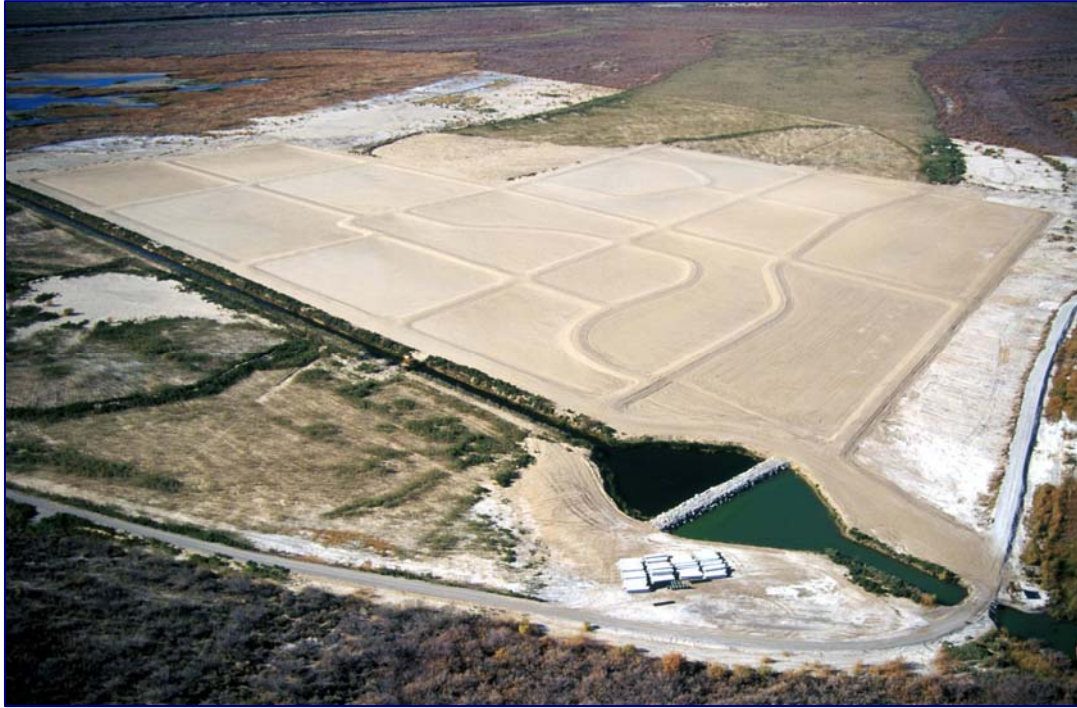
Figure 1. Aerial photo taken in 2003 as area is being divided into individual cells using berms.
