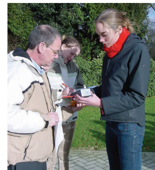
A GLOBE teacher and students learn how to measure aerosols with a hand-held sun photometer.
