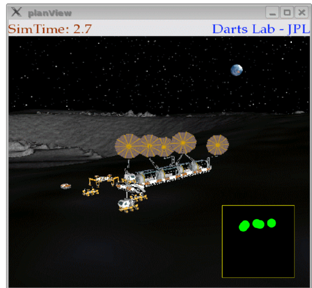
Figure 10. LSOS simulation of a potential lunar habitat system from NASA LaRC with inset Sun vector power analysis rendering.
