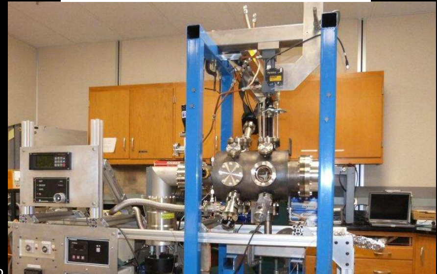
Large-Area Psec Photo-Detectors Dean Walters Bob Wagner Argonne National Laboratory Marc Kupfer University of Illinois of Chicago Vacuum Vessel for Indium cold seal.
