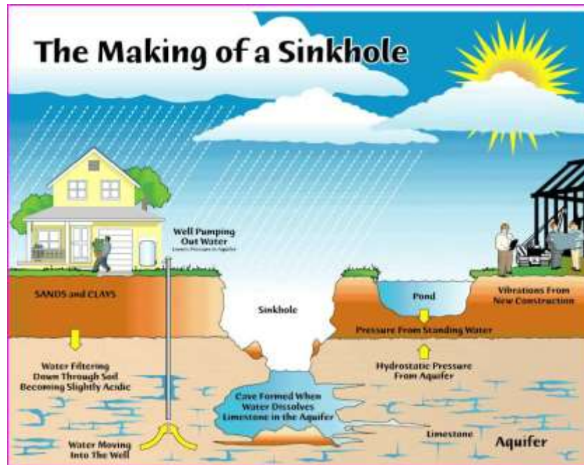
Figure D-9. The Making of a Sinkhole
