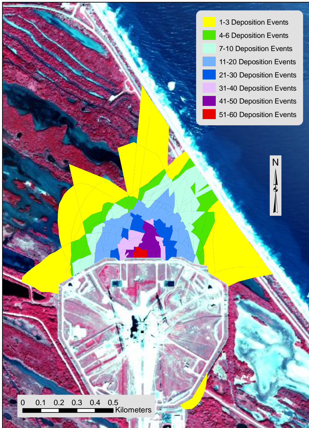
Figure 47. Cumulative near-field exhaust deposition pattern at Launch Pad 39B resulting from the solid rocket motor exhaust mixing with the deluge water (n = 53). Direction and distance of travel is controlled by surface wind speed and direction.
