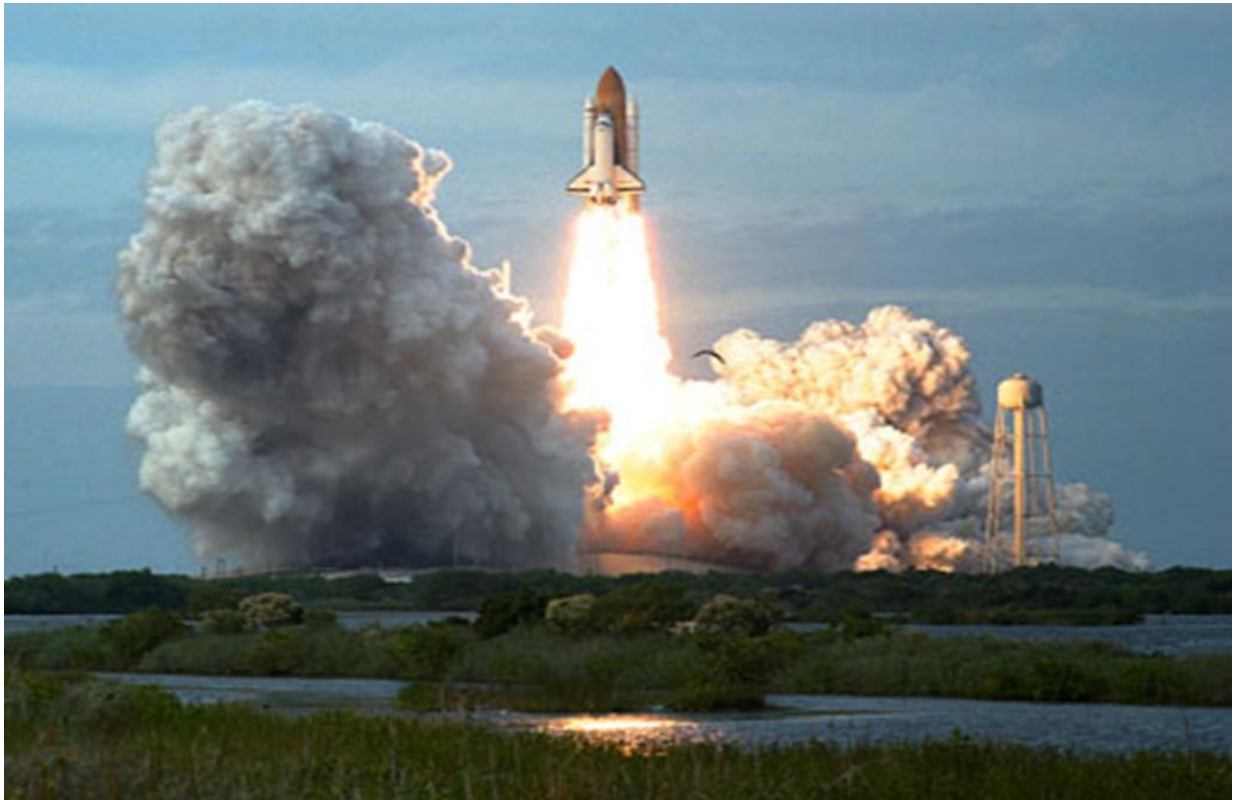
Figure 40. During the first 10-12 seconds of the launch event the Space Transportation System produced a ground cloud consisting primarily of water vapor, HCl, and aluminum oxide particulates.
