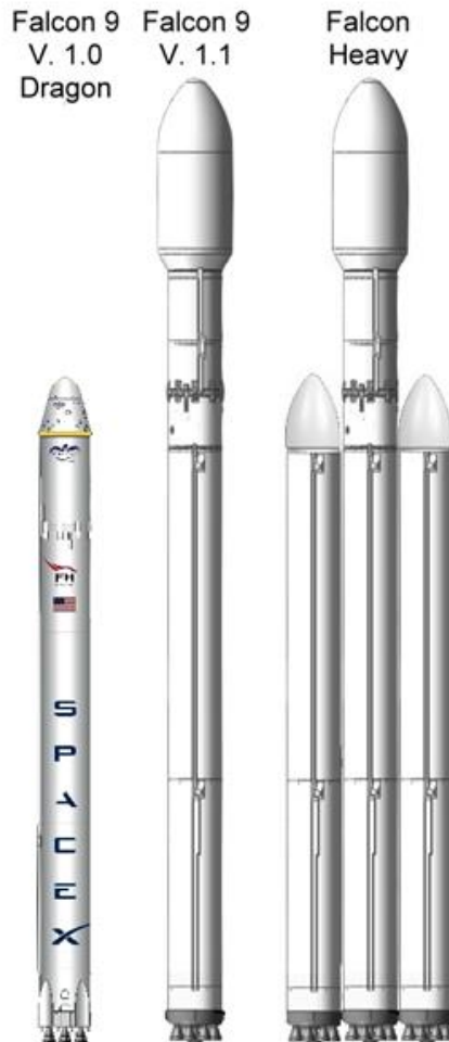
Figure 2-4. Falcon 9, Falcon 9 v1.1, and Falcon Heavy launch vehicles.
