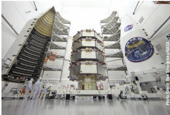
The four MMS spacecraft observatories are processed for launch in a cleanroom at the Astrotech Space Operations facility in Florida. The ambitious mission may not have happened without a handful of Goddard-developed technologies.
