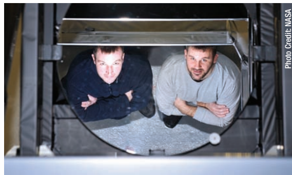
Technicians Alex Schaeffer (left) and Eric Norris (right) are seen reflected in a 3.3-foot-diameter parabolic mirror suspended 24 feet above the ground. The mirror provides a parallel beam that allowed the team to co-align NICER/SEXTANT's 56 X-ray optics.
