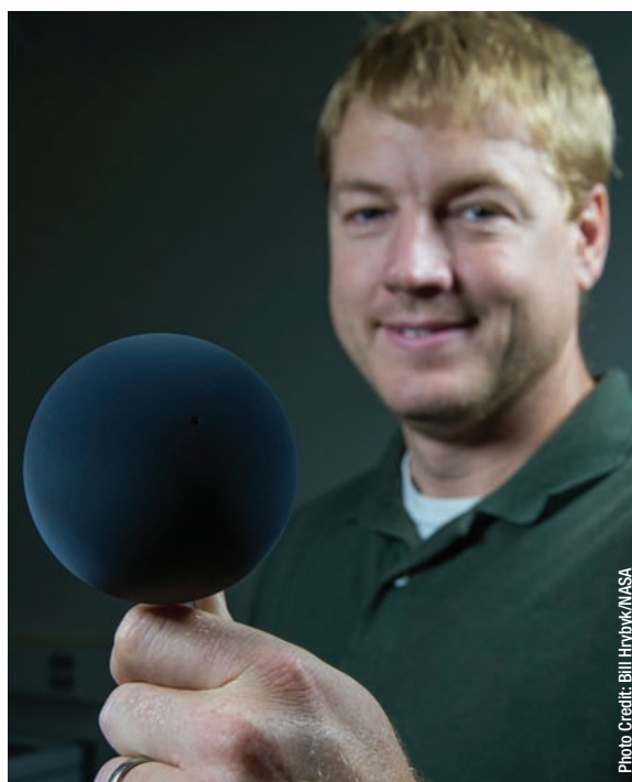
Principal Investigator Phillip Chamberlin holds a sphere coated in carbon nanotubes that he would like to fly as part of a CubeSat mission to image the sun's corona.
