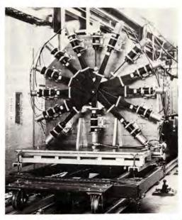
...Transmission counters used in measuring total cross sections...
