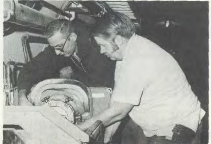
....Jack Johnson (R) places a precision cutting tool around the vacuum tube preparing to open the tube for inspection, while Tony Rader assists....
