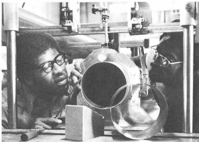
Carl Penson (left) and Ed Simmons are cutting cryostat tubes to length. Five tubes of different diameters fit inside one another to make a cryostat.
