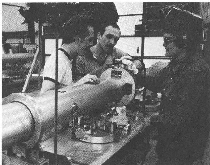
(From left) Barry Priest, Luis Torres and Violet Ball are installing suspension brackets into the cryostat to keep the tubes concentric.
