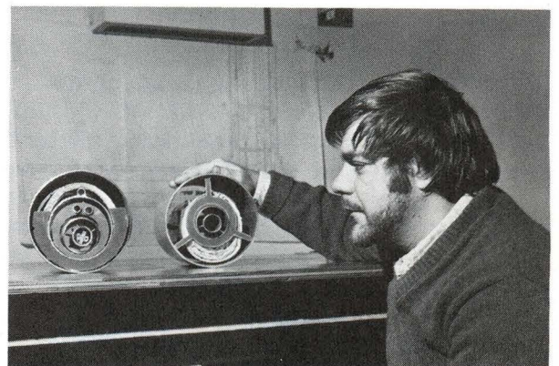
...Don Richied with cross sections of helium transfer line for doubler. Final version at left...
