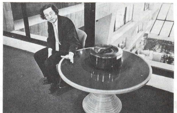
...A. Brenner, computing department head, shows magnetic disc turned tabletop and new disc pack with 50 times more data capacity...
