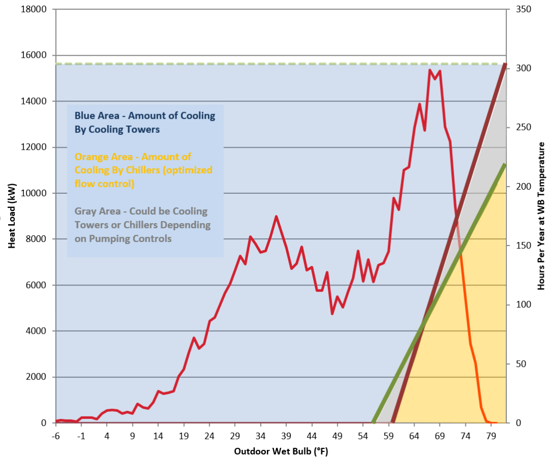
OLCF-4 Cooling Source vs Wet Bulb
