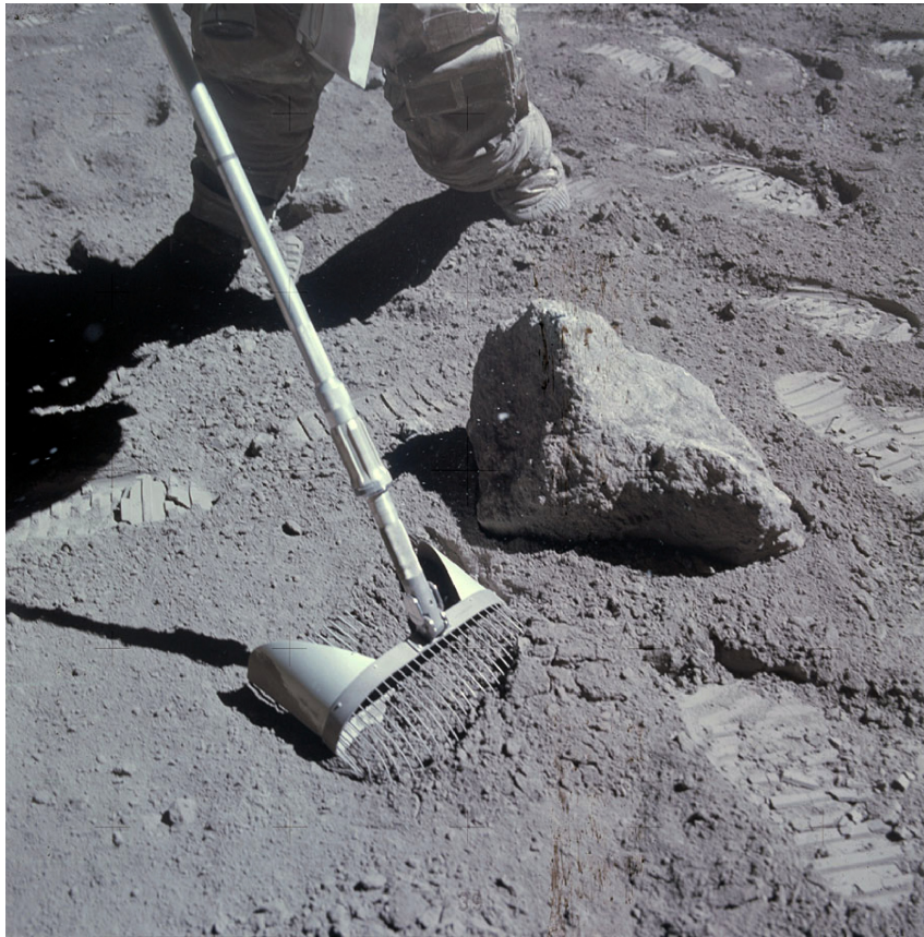
Figure 15. Collection of a rake sample on the Apollo 16 mission (Apollo 16 photograph AS16-116-18690).
