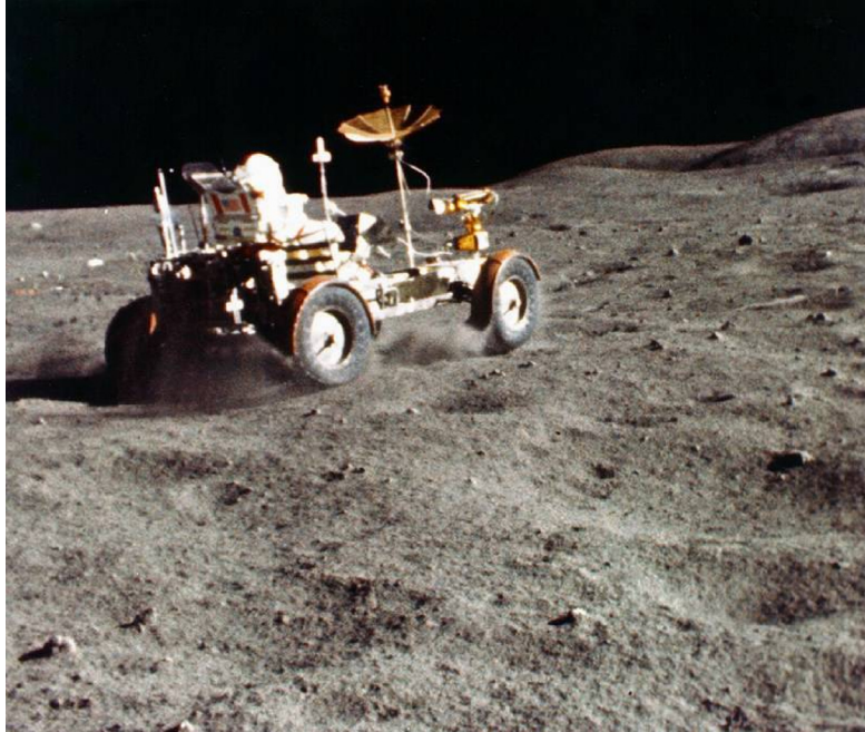
Figure 27. The LRV during locomotion. Lunar dust was frequently lifted by the wheels and deposited over the LRV (Apollo 16 photograph AP16-S72-37002).
