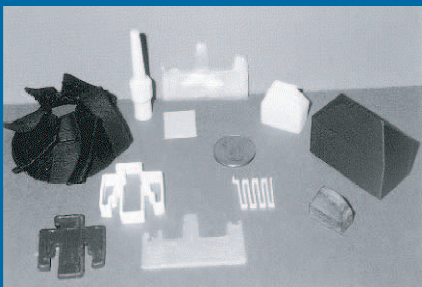
Range of objects produced by SFF deposition. Included are (clockwise from left) carbon-fiber composite turbine blade, a zirconia oxygen sensor, hydrogel, alumina, silicon carbide, silicon nitride houses. Sandia National Laboratories Thunderbird logos were prepared from alumina and Hershey's chocolate (lower left).
