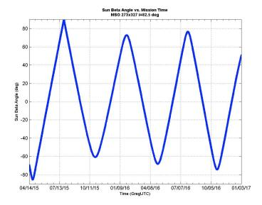
**Figure 4:** The solar beta angle versus mission time for an MSO at 273x327 km orbit and 82.5° inclination
