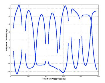
**Figure 3:** Depicts the FTIR instrument latitude access from a 273x327 km orbit, 82.5° inclination over one Martian year.
