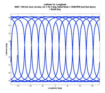
**Figure 2:** The MSO ground tracks during 1 Earth day for a near-circular orbit at ~ 300km, inclination = 82.5° and initial node = 3AM/3PM, (not Sun-synchronous). Each day accommodates approximately 13 revolutions.
