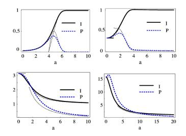
FIG. 4. (Color online) Current (plain line) and noise (dashed line) as a function of the oscillation amplitude for different values of  $\Gamma$ . From the top-left pannel  $\Gamma$ =0.001, 0.1, 1, 5. The dashed light lines are obtained with the analytical approximation (29). The short lines at a=0 are the static results given by (15).
