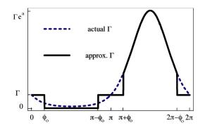
FIG. 3. (Color online) Exact and approximate dependence on  $\phi$  of  $\Gamma_L$  used to obtain analytically the FCS in the large oscillation limit.  $\Gamma_R(\phi)$  has the same form shifted by  $\pi$  in the  $\phi$  axis.
