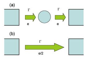
FIG. 2. (Color online) The two equivalent systems for the statistics of charge transferred in the long measurement time limit: (a) single electron transistor with equal probability  $\Gamma$  of hopping from the left lead to the grain and from the grain to the right lead; (b) a fictitious system of charges 1/2 that tunnel with probability  $\Gamma$ .
