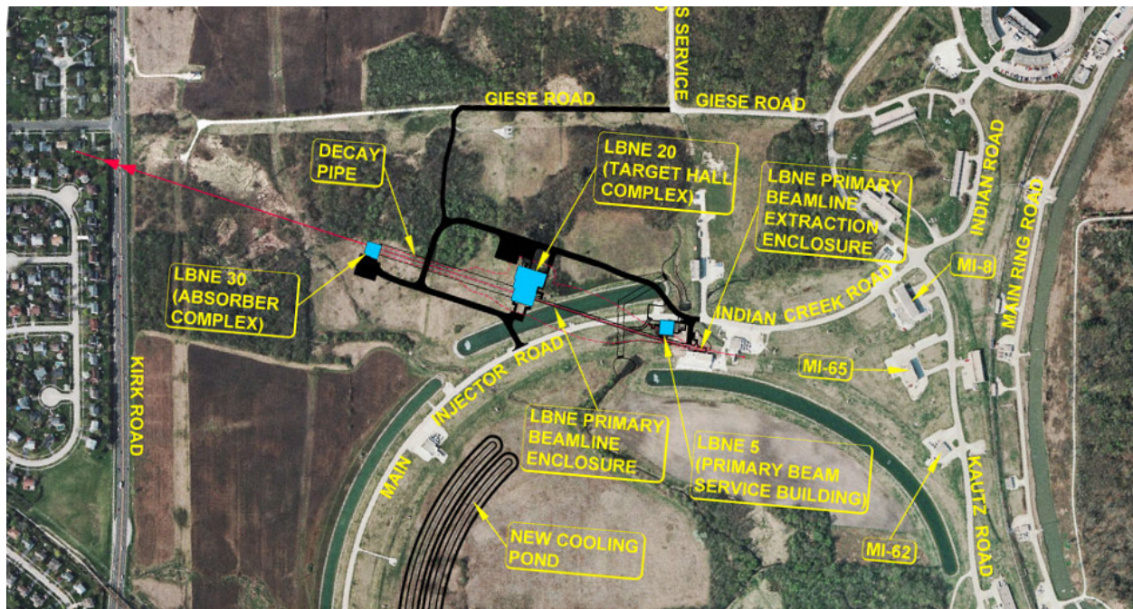
Figure 1-8: LBNE Overall Project Layout at Fermilab
