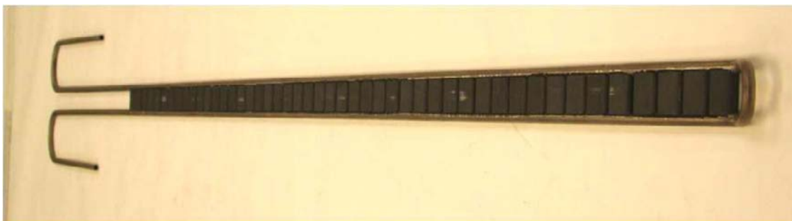
Figure 3-10: Early prototype of a target graphite core bonded to a titanium cooling line.
