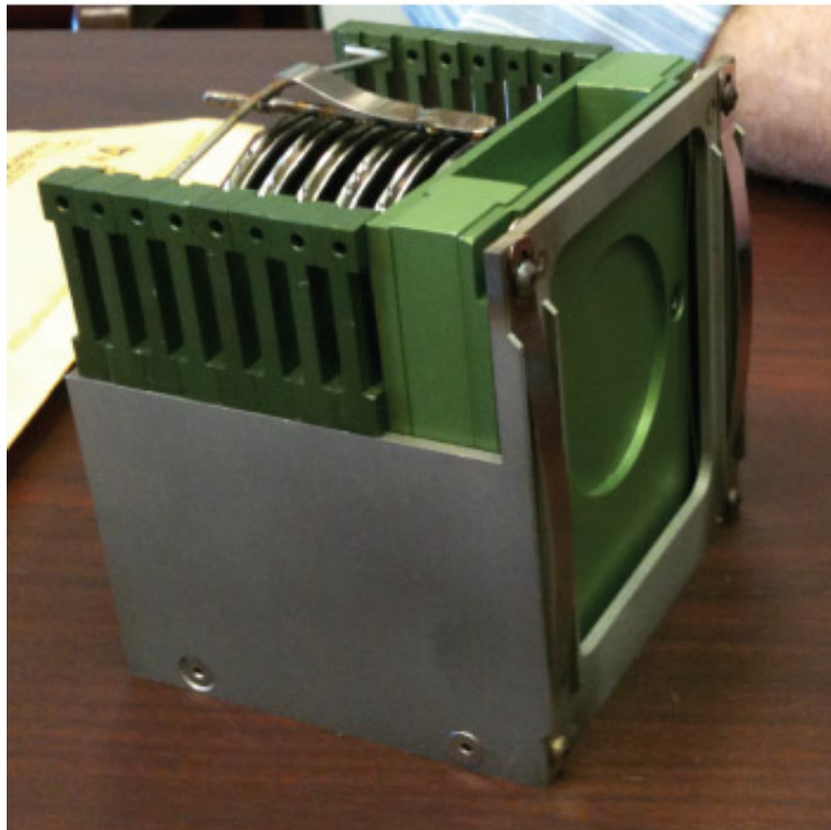
Figure 3–11: BLIP test sample holder. This figure shows cassettes of material samples irradiated in the BLIP facility. The beam enters from the right.
