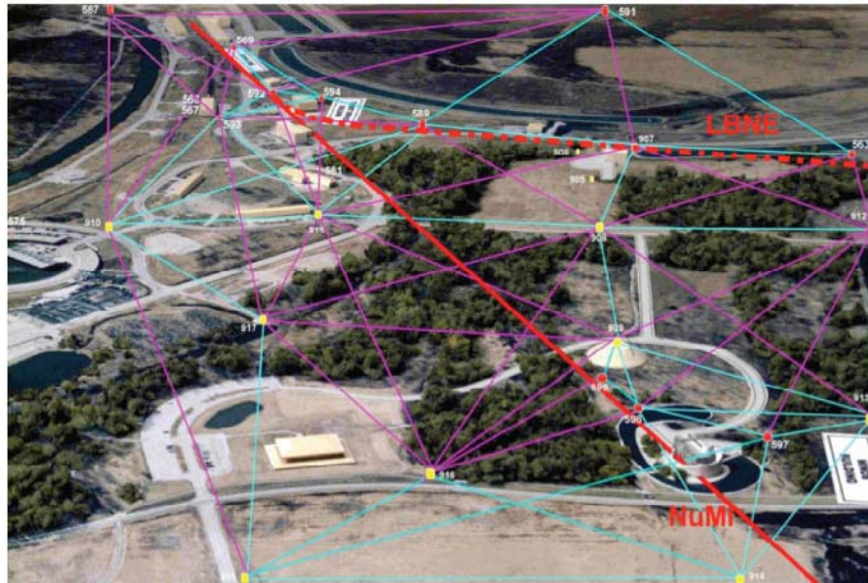
Figure 4-3: Fermilab LBNE surface geodetic network.
