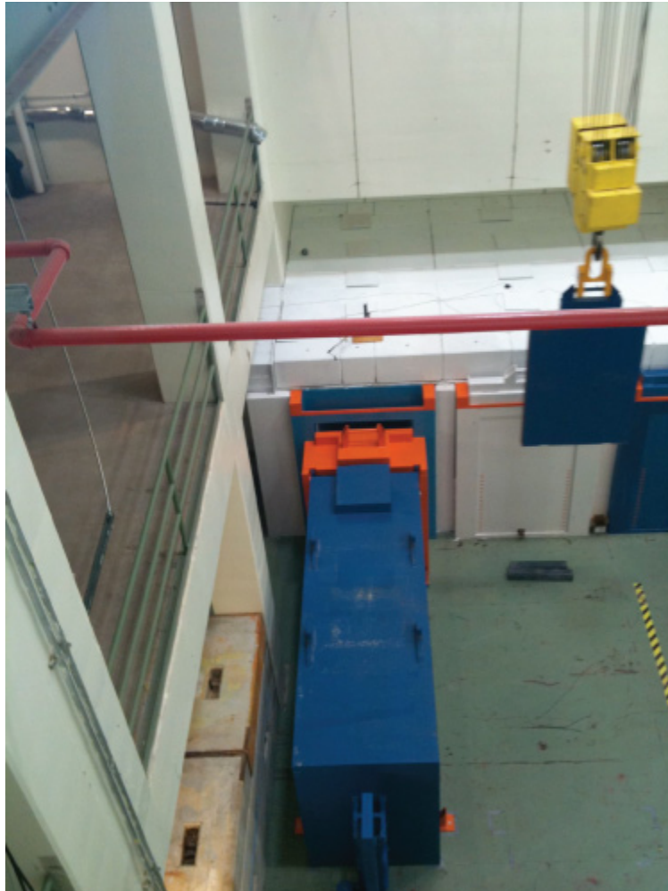
Figure 3–52: Photo of cask-to-morgue cell transfer system used at C-0 Remote Handling Facility
