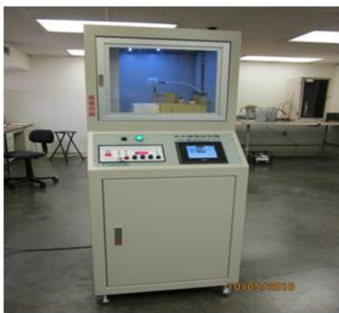
Figure III- 53: A custom-designed lab-scale electro-spinning equipment
