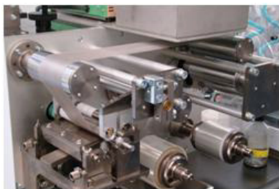
Figure III- 44: Yasui coater set up to use the micro-gravure method to apply SLMP onto a substrate.
