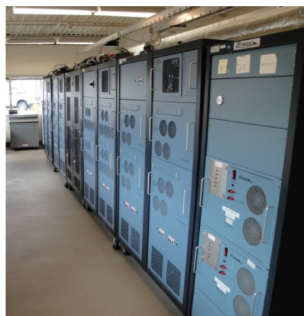
Figure II- 10: Bitrode Battery Testing Equipment at NREL’s New Battery Thermal Test Facility
