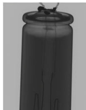
Figure IV- 149: X-ray image of an 18650 cell with an internal heater.
