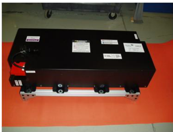
Figure III- 126: JCS 344-Volt Battery Pack
