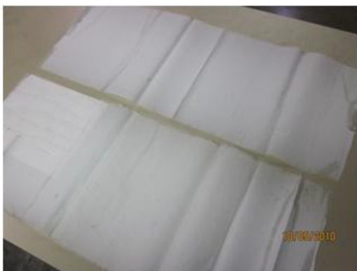
Figure III- 54: Large-format PAN nanofiber mat prepared by the new electrospinning machine
