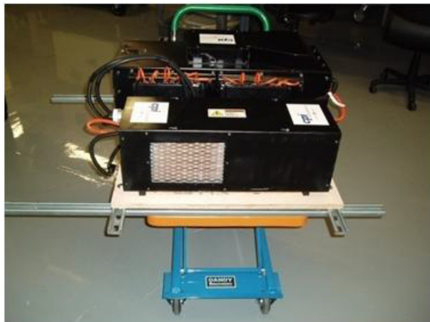
Figure III- 128: CPI 400-Volt Battery Pack
