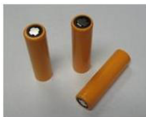
Figure III- 77: 18650 cells containing Si/C nanofibers as anodes.
