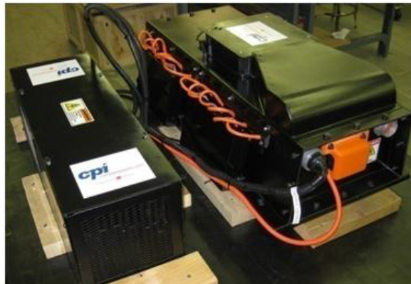
Figure III- 11: Picture of a Li Ion battery pack comprising a refrigerant-to-air cooling system and delivered to National Labs.
