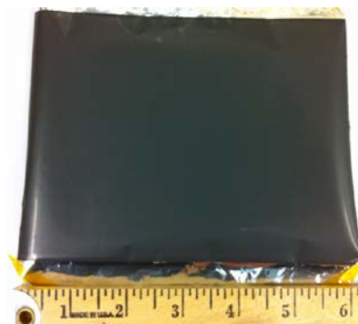
Figure IV - 65: A 6" by 6" foil of Toda HE5050 following coating with 5 cycles of ALD alumina.
