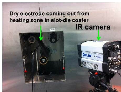
Figure IV - 87: In line IR imaging set-up on a slot-die coater.
