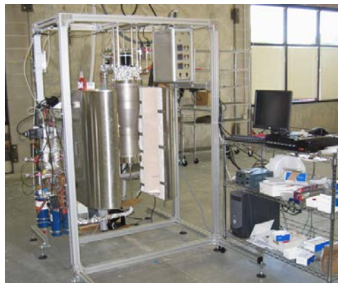
Figure IV - 69: Fluidized Bed Reactor to coat powders with ALD cycles: the existing reactor at ALD Nanosolutions can process up to 8L of powder per batch.
