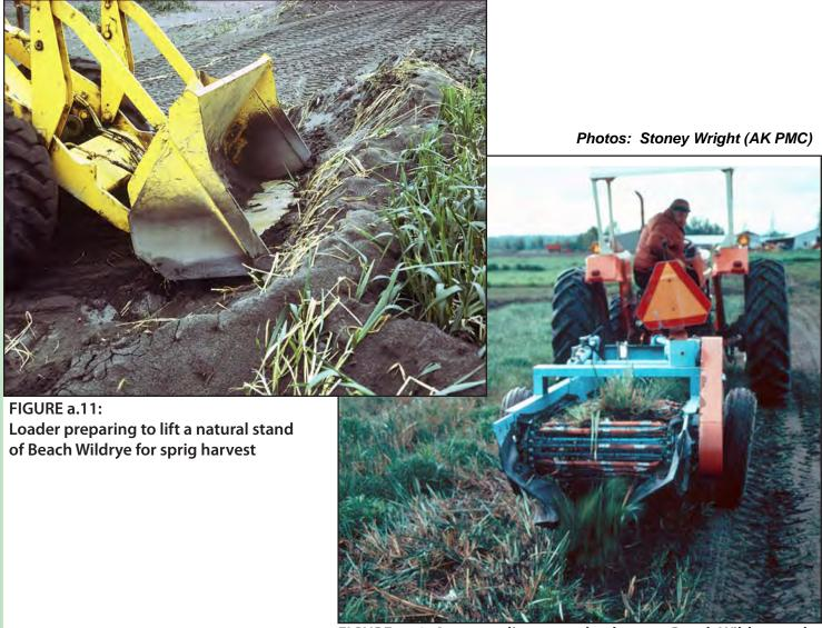
FIGURE a.12: A potato digger used to harvest Beach Wildrye at the Alaska Plant Materials Center
