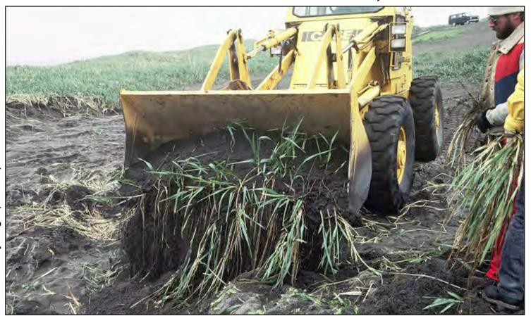
FIGURE a.10: Loader used to harvest sprigs
