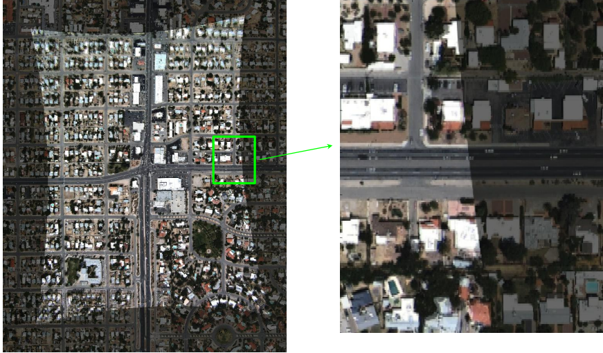
Figure 1. This shows a frame of imagery taken from the helicopter transparently superimposed over a region of the same image acquired from GoogleMaps. The region in the green box on the left is shown zoomed in on in the image on right. The irregular boundaries of the image are due to the radial distortion correction and registration processes.
