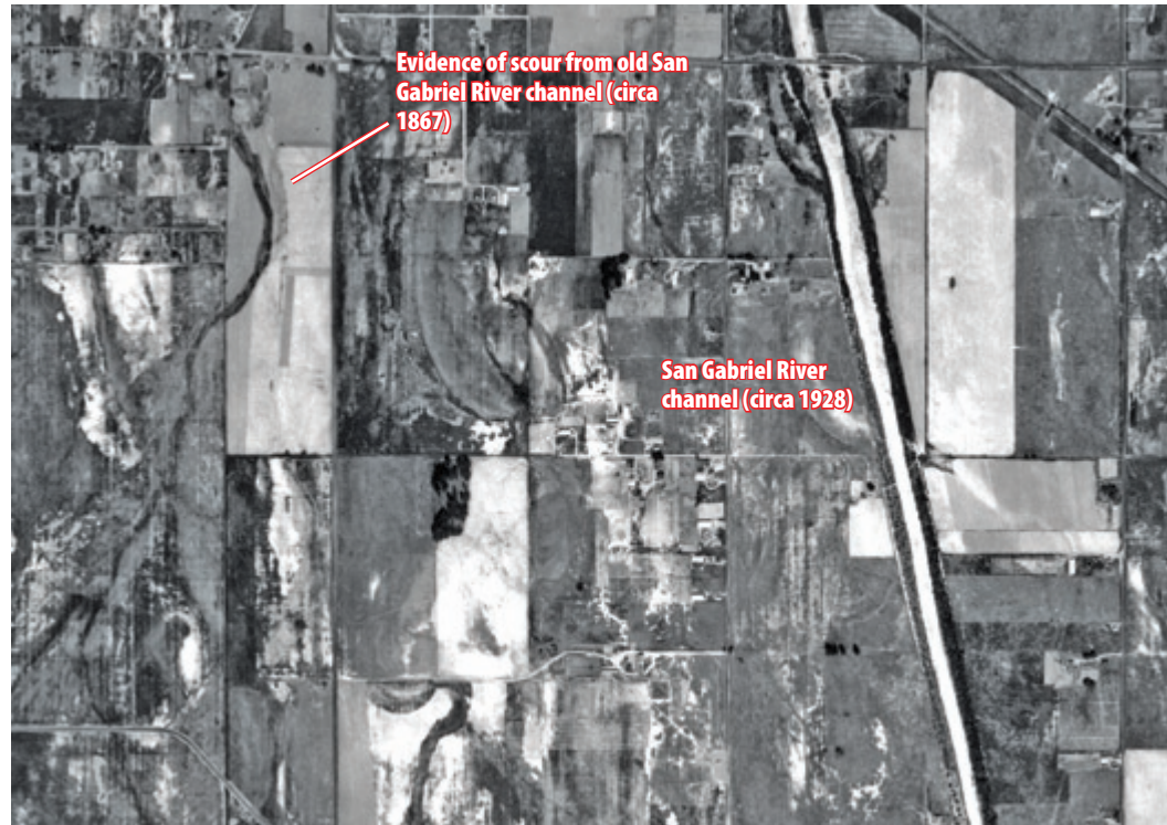
FIGURE 3.7. Aerial photograph showing the channelized San Gabriel River in 1928, as well as evidence of a previous channel. The photograph also provided further collateral data on the size of the southern San Gabriel River flood plain.
