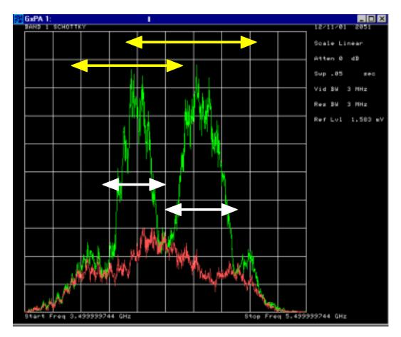
Debuncher Band 1 Momentum Signal to noise. Yellow Arrows top indicate current filter bandwidths. Low band 3.8-4.6 Ghz; high band 4.2-5.1 GHz White Arrows bottom indicate desired filter bandwidths Low band 4.0-4.5 GHz high band 4.5-5.0 GHz
