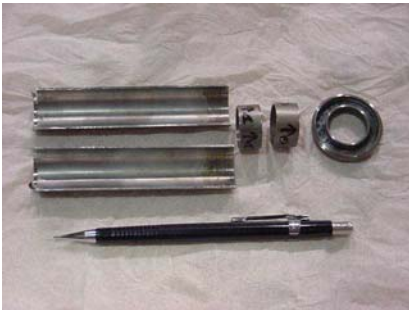
Photo 13 – Lens 18 inner conducting tube after sectioning
