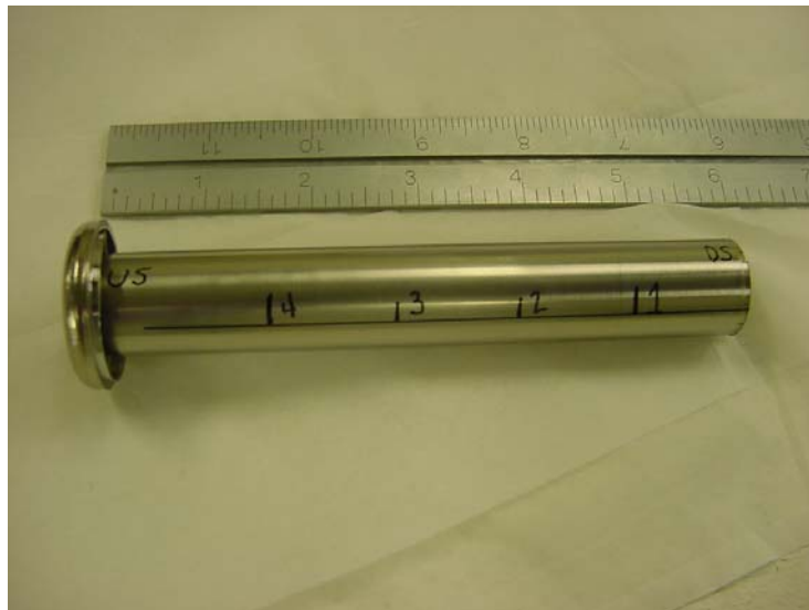
Photo 14 – Lens 16 inner tube removed from septum prior to sectioning
