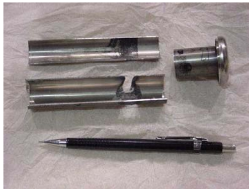
Photo 10 – Lens 17 inner tube after sectioning
