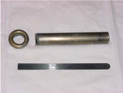
Photo 11 – Lens 18 inner conducting tube removed from septum
