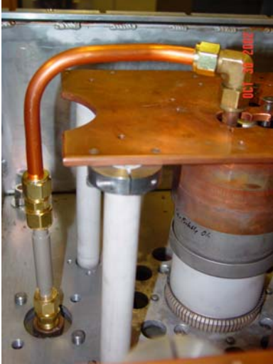
Close view of the modified water connections. Much better than the hose type DC block. Also note the ceramic (this case picture) standoff set to 8.5 inches. Careful!
