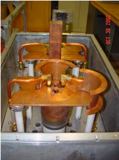
Wide view of amplifier. Notice the \frac{1}{4} inch spacers screwed onto the frame. No touch!
