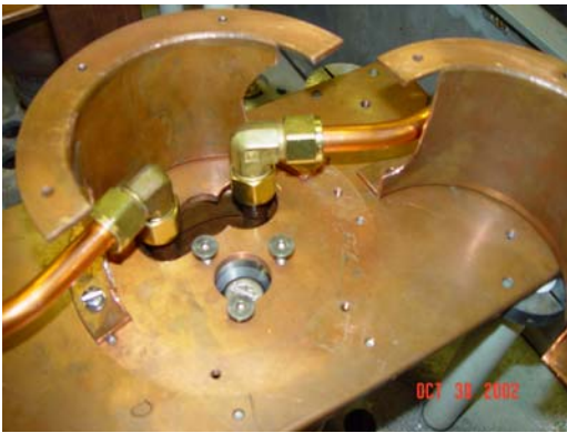
Notice the split spacers used to access the water connections at the tube. Also the three screws on the clamp assembly used to push against the tube collar ring to keep it snug when in its operating position.
