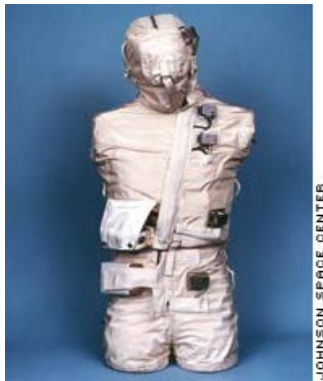
Fig. 2. The JSC phantom torso as flown on STS-91 [Cucinotta 2004].
