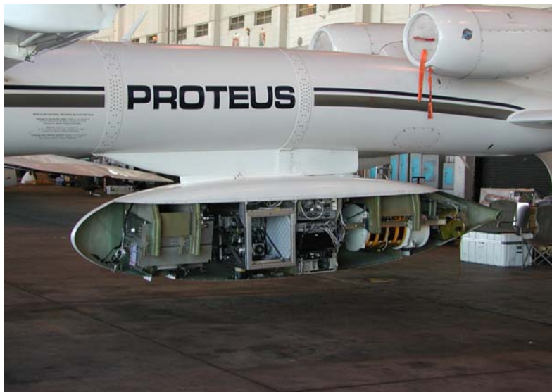
Figure 22 A UAV platform, Proteus, that has the potential to carry a RAOBS system.
