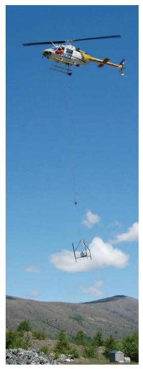
On July 14, 2009, several "spider" pods like the one shown above were lowered by cable from a helicopter hovering about 100 feet up and gently put in hot spots inside and around the volcano crater of Mt. St. Helens. (Image Credit: Willie Scott / USGS)
