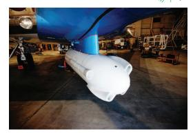
Above, the UAVSAR (Uninhabited Aerial Vehicle Synthetic Aperture Radar) pod below the NASA Gulfstream III aircraft. Developed with ESTO funding, UAVSAR is now a fully-operational airborne instrument for surface deformation measurements. ESTO is currently conducting studies to integrate the technology onto the Global Hawk UAV platform. (Image Credit: Dave Bullock, Wired.com)
