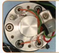
The Advanced Accuracy Satellite Instrumentation for the CLARREO Mission project seeks to develop and test several key calibration subsystems, such as temperature calibration for the blackbody cavity shown at left, dual absolute radiance interferometers, and an emissivity module. (PI: H. Revercomb, University of Wisconsin)
