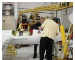
Above, one of the two INFLAME instruments is mounted in the wing tip tank of the Learjet aircraft. (Image courtesy Marty Mlynczak)
