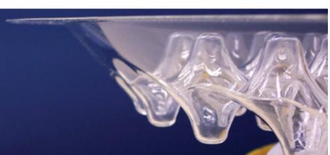
in months to years and millions of dollars. This ACT project (PI: R. Egerman, ITT Geospatial Systems) demonstrated a new approach to mirror fabrication using borosilicate, an inexpensive and easy-to-work glass to develop new mirror designs.
