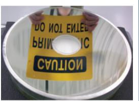
Above, one of the 0.5m mirrors shown with a spray-silver coating after final polishing and ion figuring. (All images courtesy ITT Geospatial Systems)
