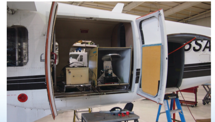
Right: The WISM instrument being integrated into the Twin Otter Aircraft. Below Right: The Twin Otter gets a final checkout on the first day of flights. Below: The ground crew takes a break. Ground observations were carried out on Grand Mesa along the WISM flight line and included 19 detailed snow pits (snow density, temperature, grain size, grain type, layer thickness profiles), 8,000+ manual depth measurements, and two snowmobile-based radars that profiled the entire line multiple times at 10 cm resolution. (Credit: Tim Durham, Harris Corp.)
