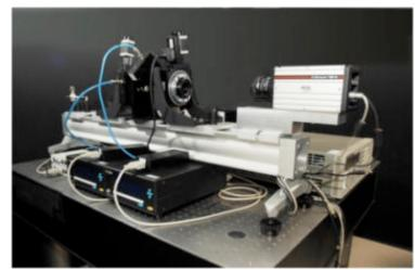
PolZero polarimeter testbed
