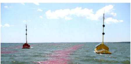
Telesupervised Adaptive Ocean Sensor Fleet investigating a Harmful Algal Bloom (simulated with water-tracing dye).
