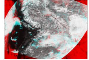
Automatic registration between images taken 100 minutes apart with the Moderate Resolution Imaging Spectroradiometer (MODIS) instrument on Aqua (cyan) and the twin MODIS instrument on Terra (red).
