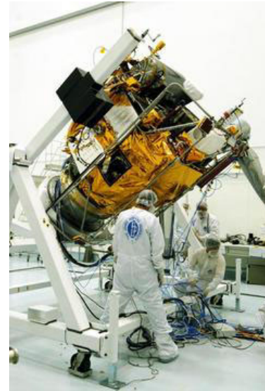
At the Astrotech Space Operations facilities near KSC, workers rotate the MESSENGER spacecraft on the turnover fixture to perform the propulsion system phasing test - firing gas through the thrusters to verify that the right thrusters fire when expected - as part of prelaunch testing.
