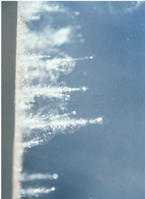
Close-up of particles captured in aerogel during an experiment using a special air gun to shoot particles at high velocities.
