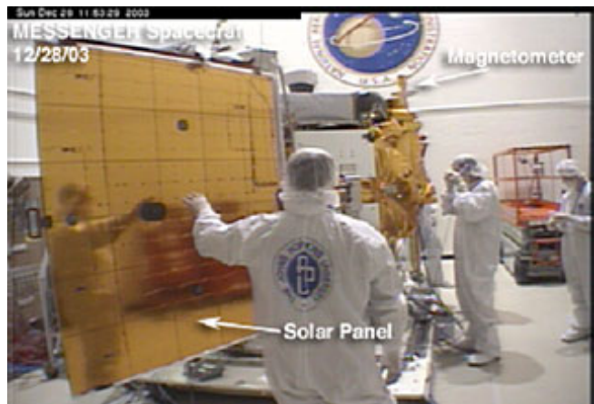
MESSENGER team members check the spacecraft after the acoustic test by deploying a solar panel, using the same type of pyrotechnically triggered separation nuts MESSENGER will use in flight. Both solar panels as well as the magnetometer boom were successfully deployed.
