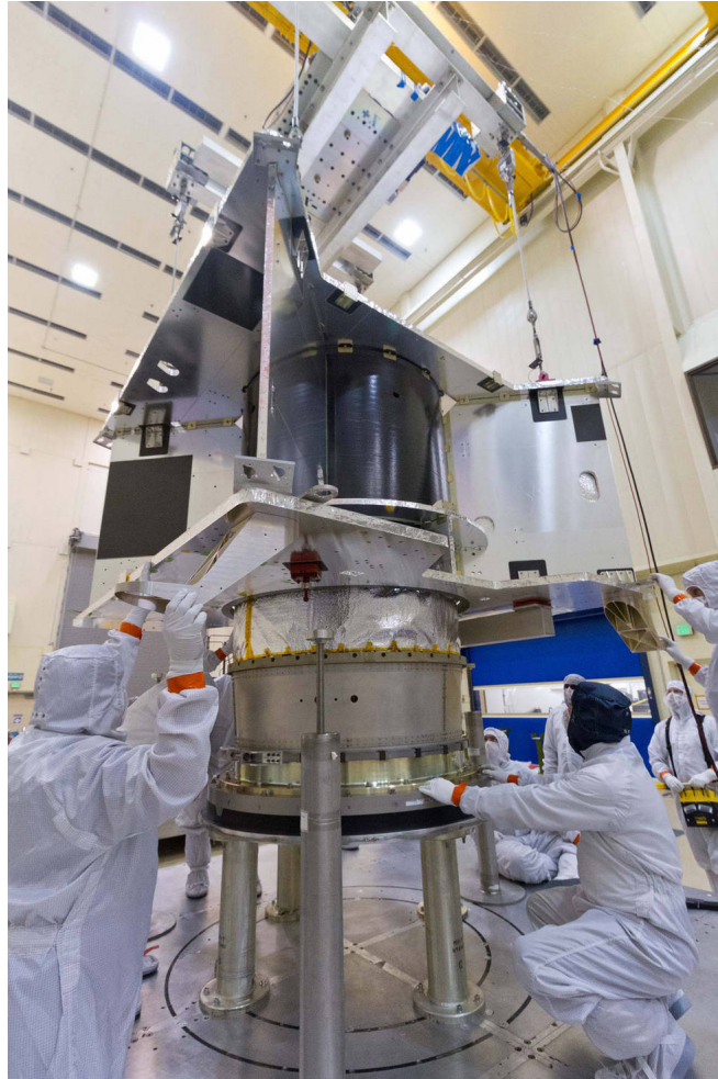
The OSIRIS-REx spacecraft core structure is successfully lowered and mated to the hydrazine propellant tank and boat tail assembly at Lockheed Martin, Denver. Credit: Lockheed Martin
