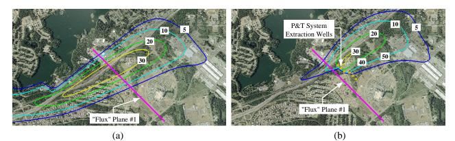
**Figure 27.** Contaminant Contours (µg/L) After 25.5 Years for the Scenarios of (A) Natural Attenuation Only and (B) Pump-And-Treat; the Pump-And-Treat System Was Discontinued After this Time
