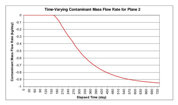
Figure 17. Plot of the Mass Flow Rate of Contaminant Across Plane #2 as a Function of Time
