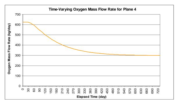
Figure 23. Plot of the Mass Flow Rate of Oxygen Across Plane #4 as a Function of Time
