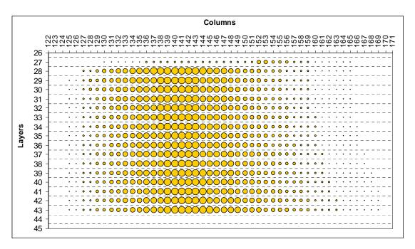
*Figure 29.* Relative Contaminant Concentration (mg/L) at Flux Plane #1 on Simulation Day 10000 of the Multilayer Example "No Action" Scenario
