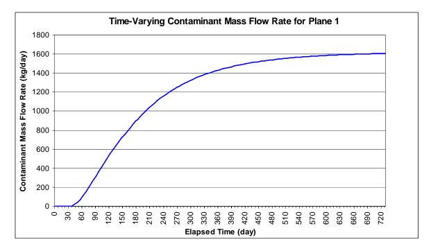
Figure 16. Plot of the Mass Flow Rate of Contaminant Across Plane #1 as a Function of Time
