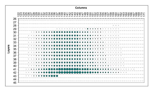
*Figure 30. Relative Mass Flow Rate (kg/day) at Flux Plane #1 on Simulation Day 10000 of the Multilayer Example "No Action" Scenario*
