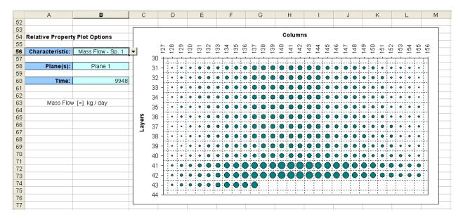
**Figure 4.** Example of a Bubble Plot Showing the Relative Magnitude of Mass Flow Rate for a Specified Plane at a Particular Time Point in the Simulation — Drop down lists allow the user to select the property (also including volumetric flowrate and concentration), plane, and time to display. The bubble sizes are scaled relative to the largest value in the simulation so that the size shows the proper relative magnitude when looking at different time points.
