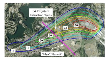
Figure 24. Plan View of the Multilayer Example Showing Initial Conditions in Layer 33, the Location of Flux Plane #1, and the P&T Wells
