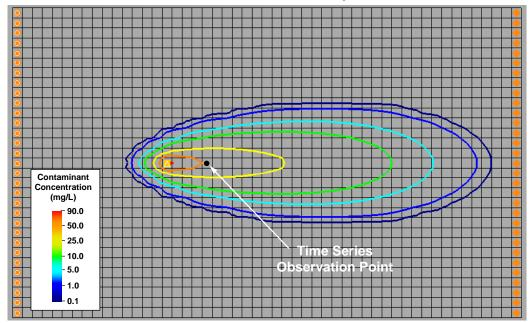
Figure 13. Concentration Contours After 730 Days for the Contaminant Component
