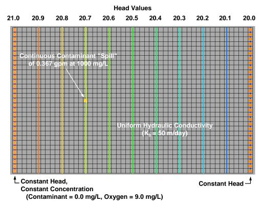
*Figure 10.* The Scenario for the Simple Example Showing the Uniform Hydraulic Gradient, Boundary Conditions, and the "Spill" Location
