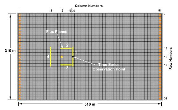
*Figure 11.* Locations of the Four Flux Planes Used in the Simple Example and the Observation Point for Time Series Concentration Plots
