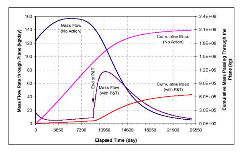
*Figure 26.* Mass Flow Rate and Cumulative Mass to Pass Through a Plane for the Two Scenarios of the Multilayer Example — In one case no action is taken (natural attenuation only) and in the other P&T is applied. In both cases, the non-aqueous phase liquid source was removed.
