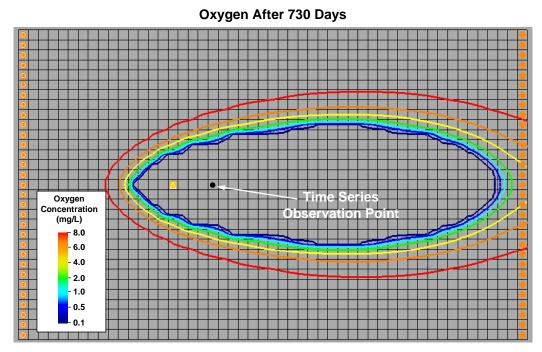
Figure 14. Concentration Contours After 730 Days for the Oxygen Component
