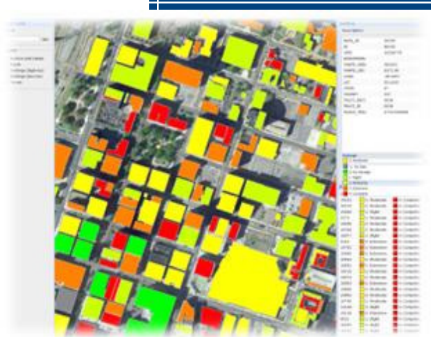
SUMMIT building adjudication tool provides an editable visualization of building damage data
