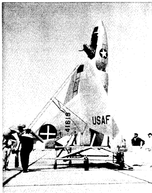
The Ryan X-13, an experimental tail-sitting testbed, represented an interesting, if unsatisfactory, attempt to develop a practical vertical take-off and landing concept.
