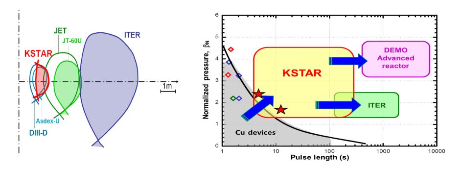
Machine design is optimized for advanced target operation Strong plasma shaping, Passive stabilizing plates, low TF ripple..
