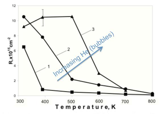
Fig. 8 Deuterium retention in 18Cr10NiTi steel implanted to  $1 \times 10^{16}$  cm<sup>-2</sup> without helium (1) and with helium to  $5 \times 10^{15}$  (2) and to  $5 \times 10^{16}$  cm<sup>-2</sup> (3).
