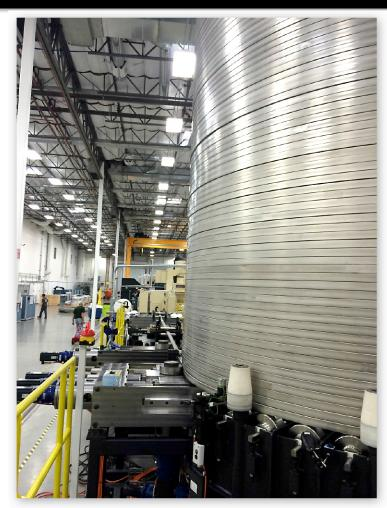
Conductor routed from the de-spooler of the winding station
