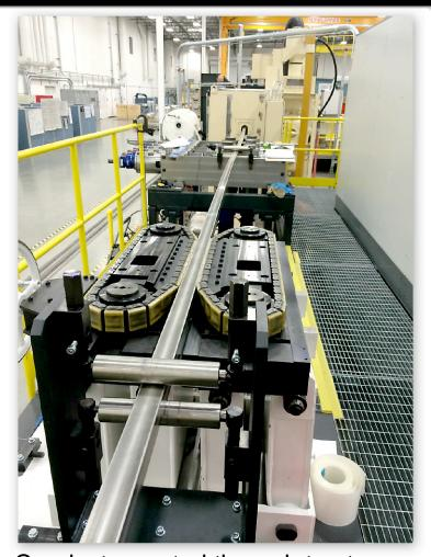
Conductor routed through tractor drive to the straightener Photos: General Atomics
