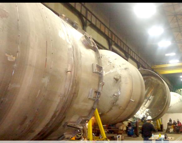
All drain tanks (four 61,000 gallon drain tanks and one ~30,000 gallon tank) will complete fabrication by February 2015. At left, a completed tank undergoes a lifting test. At right, tanks in earlier stages of fabrication.
