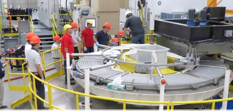
300 m double pancake coil on winding table with cleaning grit blast and de-spooler stations behind
